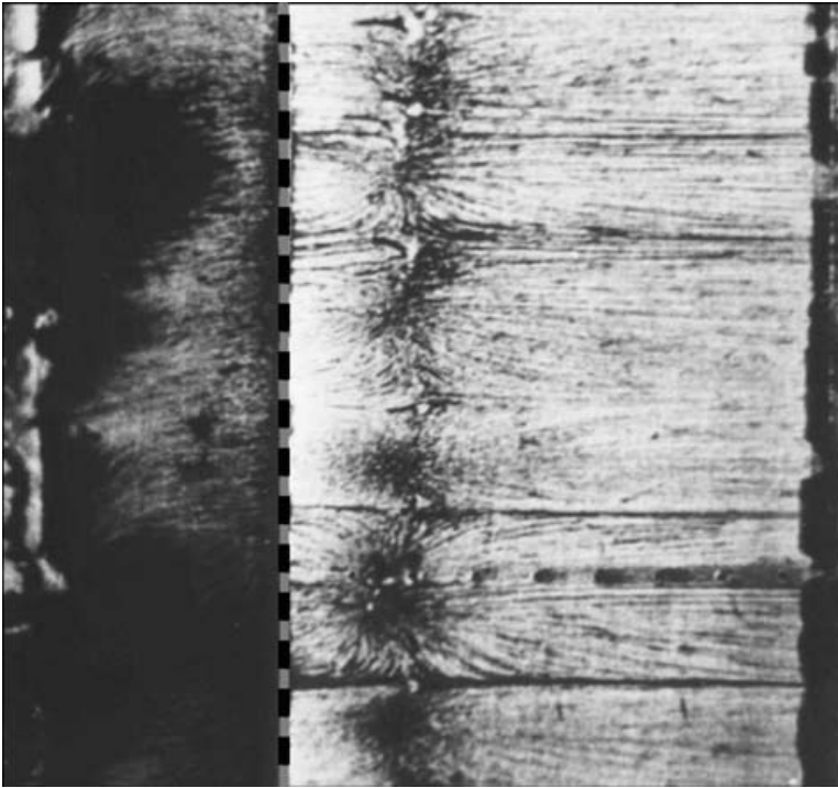
FIGURE 11. Oil-flow visualization pattern from higher-Reynolds-number experiment; the thick dashed vertical line indicates the corner position.
